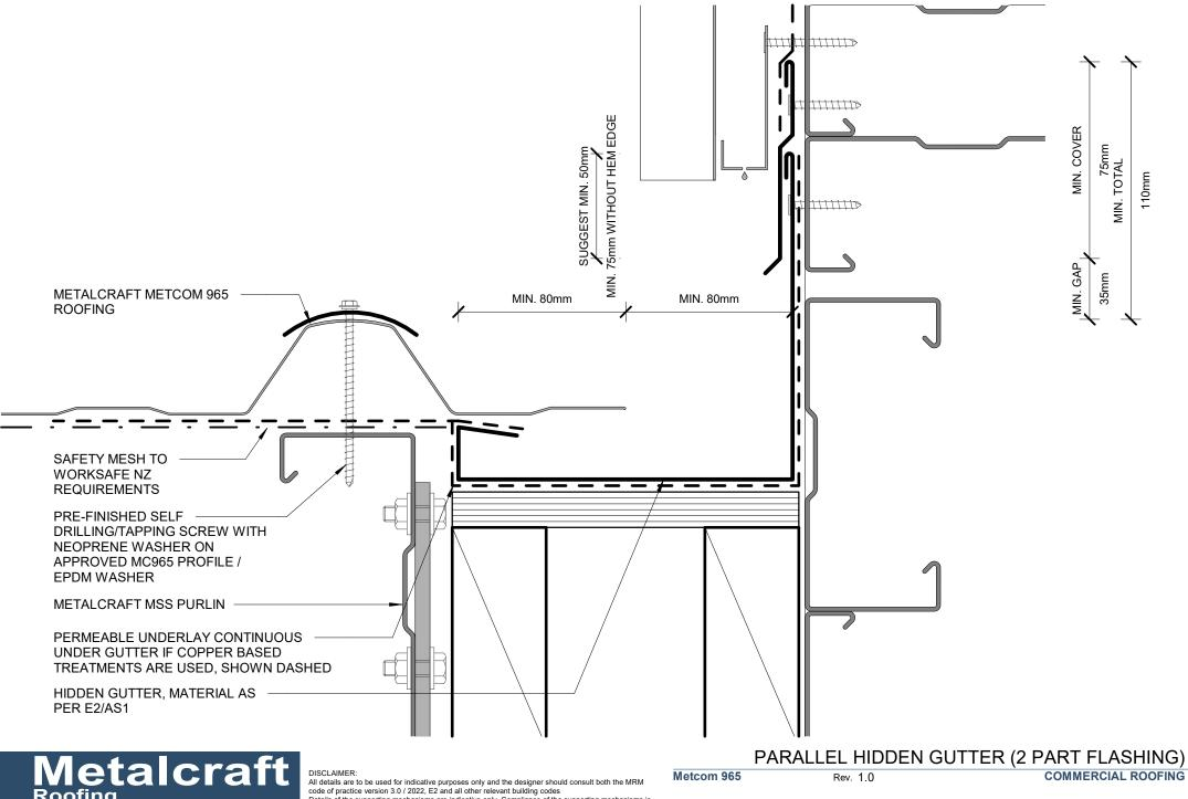
Details of the supporting mechanisms are indicative only. Compliance of the supporting mechanisms is the responsibility of the designer. Construction detail can vary for wall cladding. The underlay is detailed as a single line for simplicity and is indicative only. Building paper type and method of installation should comply with underlay manufacturers recommendations and NZBC regulations.
