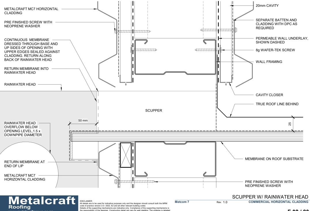
the responsibility of the designer. Construction detail can vary for wall cladding. The underlay is detailed as a single line for simplicity and is indicative only. Building paper type and method of installation should comply with underlay manufacturers recommendations and NZBC regulations.
