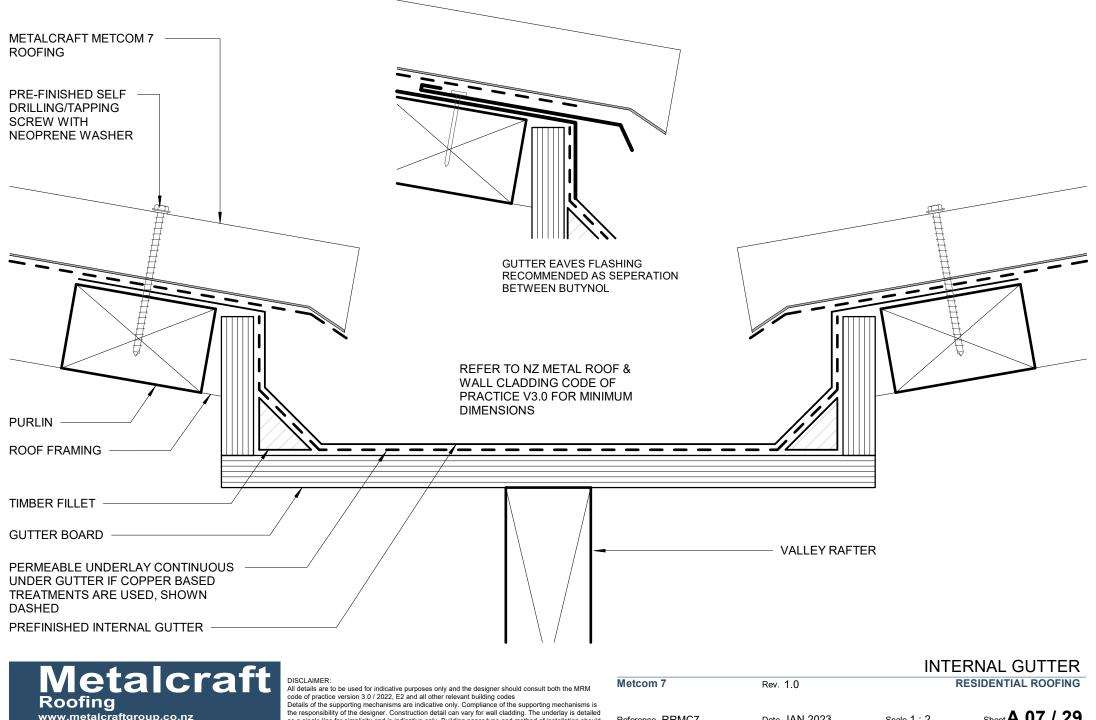
as a single line for simplicity and is indicative only. Building paper type and method of installation should comply with underlay manufacturers recommendations and NZBC regulations.
