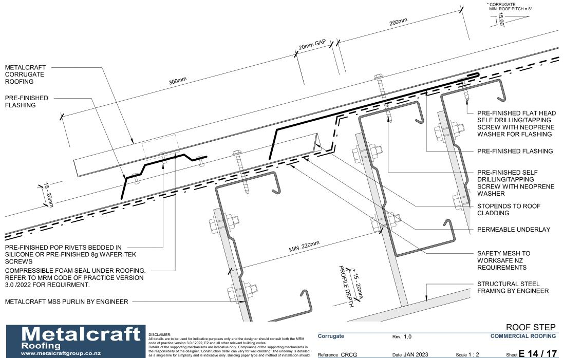
as a single line for simplicity and is indicative only. Building paper type and method of installation should comply with underlay manufacturers recommendations and NZBC regulations.
